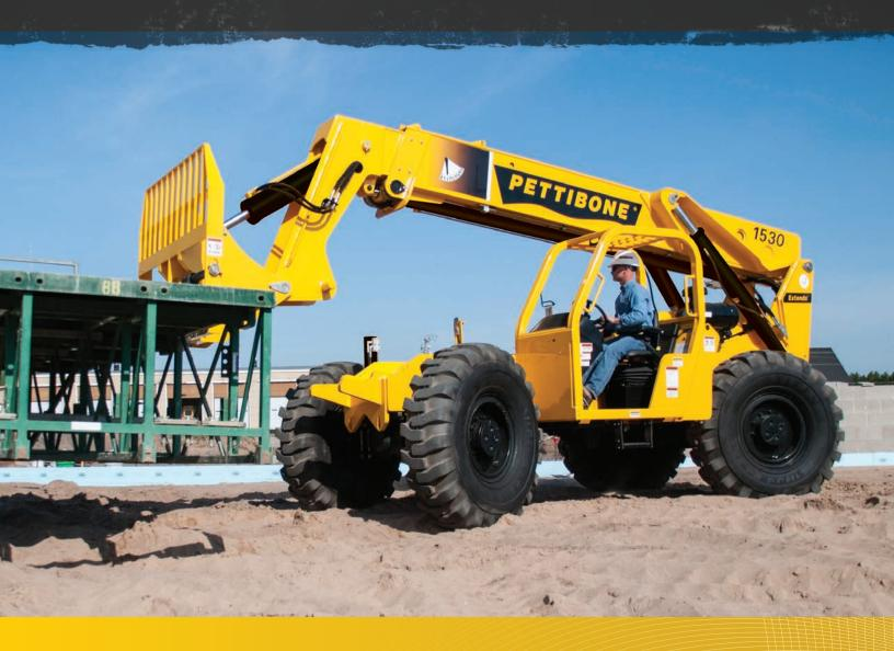
Featuring heavy-duty lift cylinders, automatic fork leveling and rear axle stabilization, the Pettibone® Extendo™ 1530 is built for productive load handling on difficult jobsites. Excellent cab visibility and a rapid response hydraulic system contribute to maximum efficiency and enhanced safety. Additionally, four-wheel drive and three steering options help provide unmatched maneuverability on the job.
