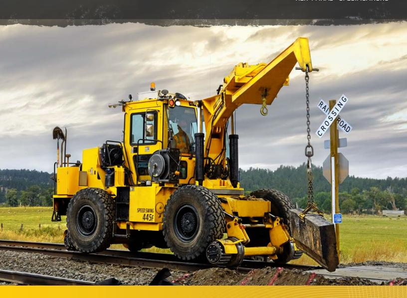
Designed to tackle a variety of rail applications, the Pettibone® Speed Swing™ 445F is a versatile machine that provides the power to lay rails, set ties or clear the path ahead. The unit features a turbo diesel engine and 180-degree boom rotation for enhanced productivity. Offering precise hydraulics, numerous attachments and the ability to work both on and off the rails, the Speed Swing 445F is equipped for any rail task.
