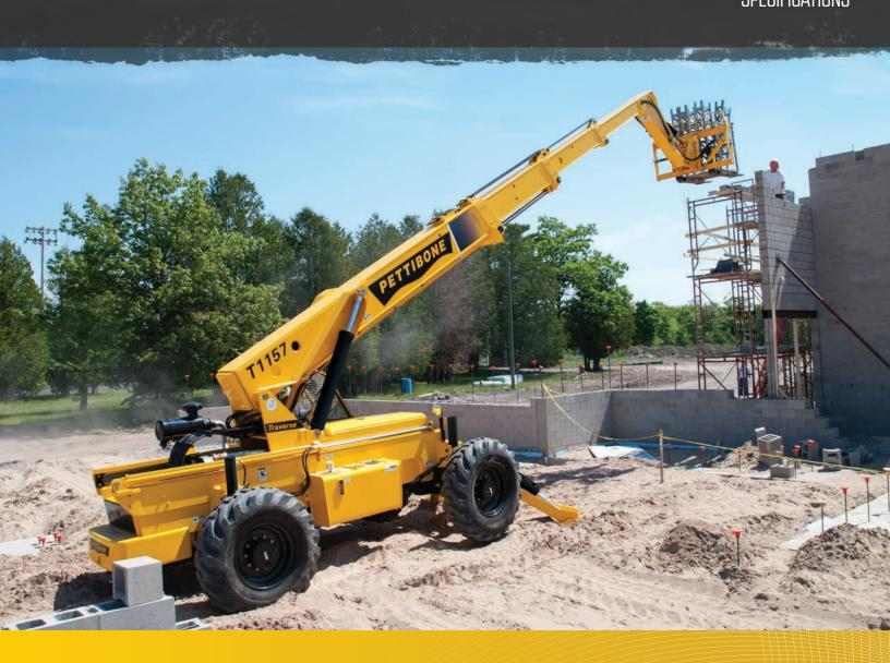
The Traverse™ T1157 from Pettibone® is ruggedly built and engineered to deliver results for the long haul. High lift capacity and reach, along with 70 inches of horizontal boom transfer, makes easy work of landing loads. The T1157 also offers exceptional operator visibility and superior maneuverability for enhanced efficiency. Responsive hydraulics ensure smooth operation for any job application.
